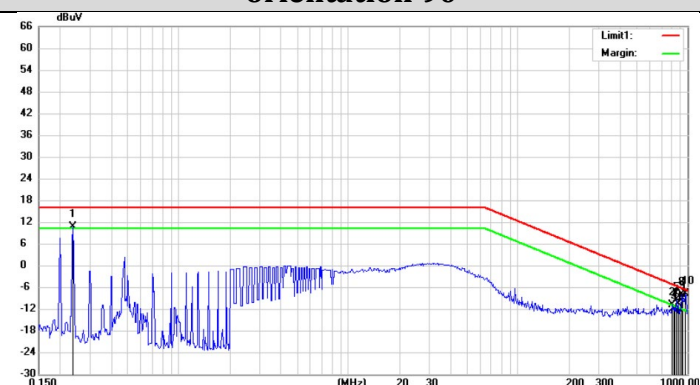
VCC1=5.5V, VCC2=33V, TTL Input 1kHz, orientation 270°
